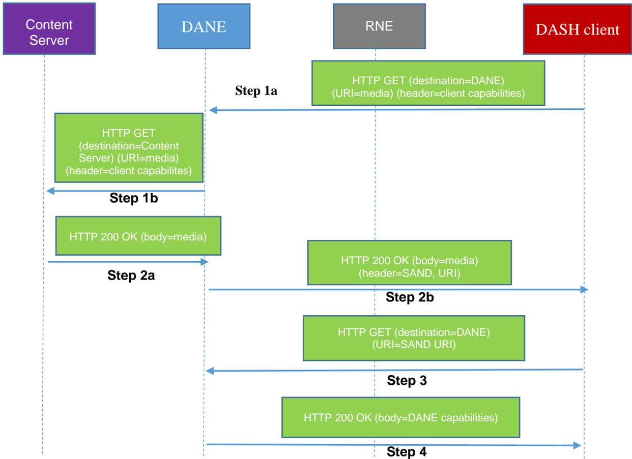
**Figure 3 - Workflow for client-triggered SAND capability exchange / negotiation.**
