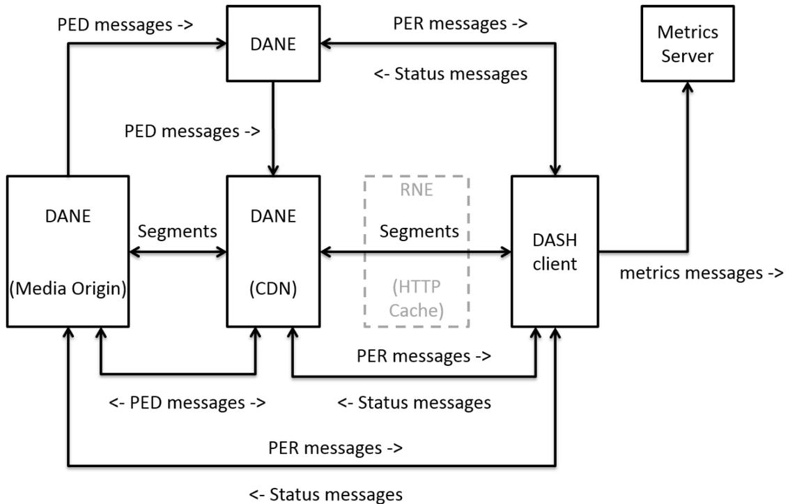
**Figure 1 - SAND reference architecture (taken from ISO/IEC 23009-5 [1])**
