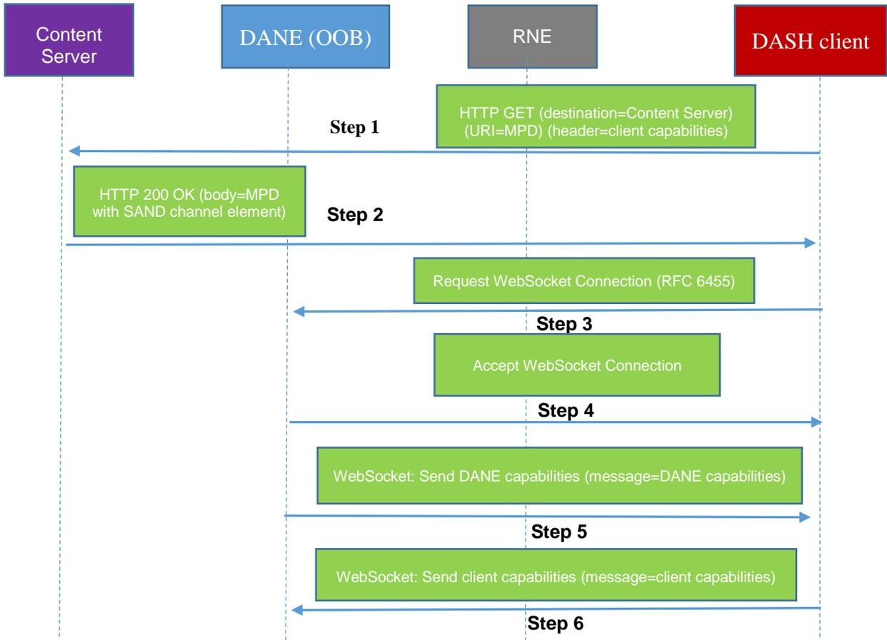
**Figure 5 - Workflow for client-triggered SAND capability exchange / negotiation using WebSocket.**
