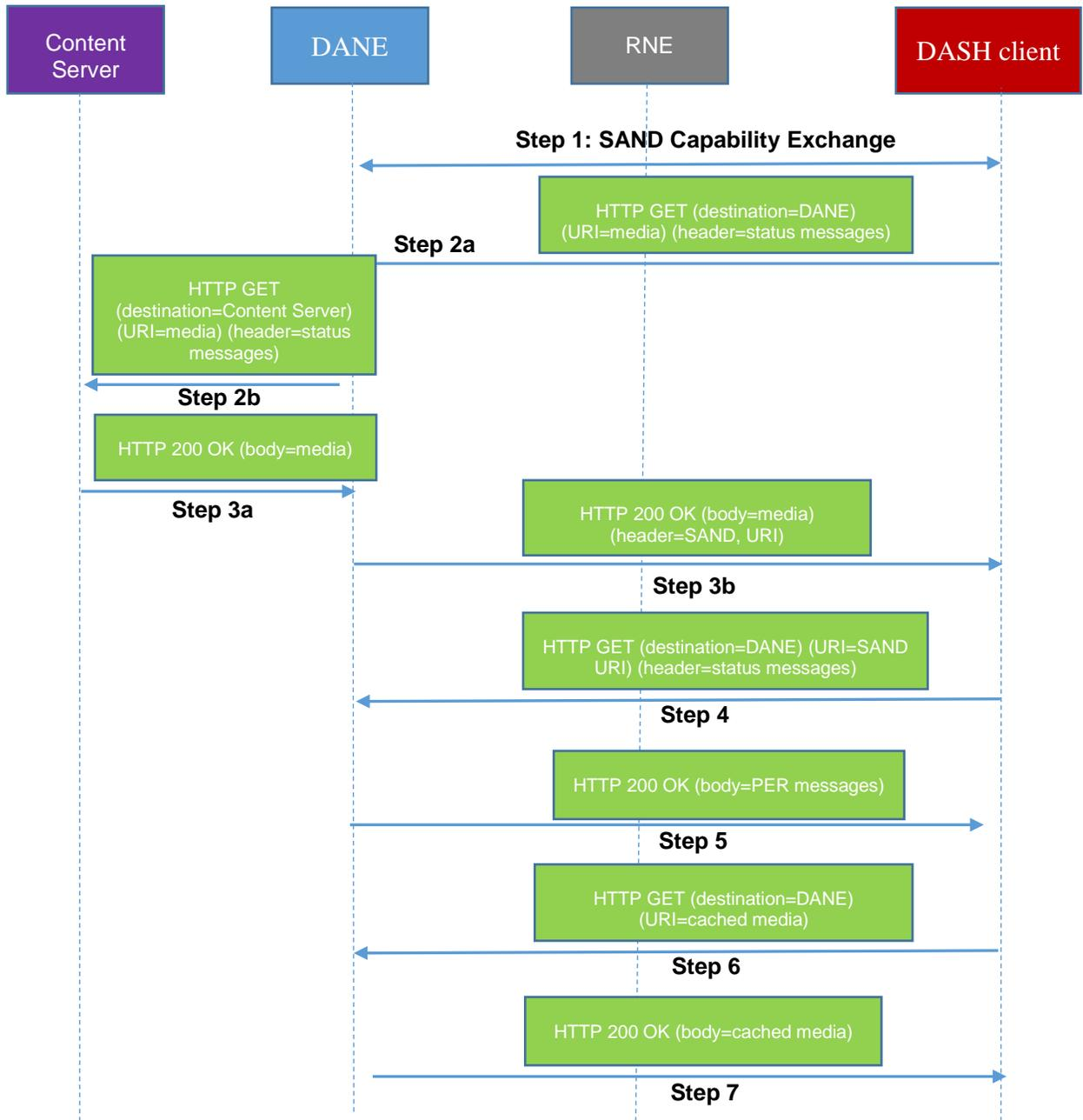
Figure 6 - Workflow for Proxy Caching for the case of on-the-fly caching.
