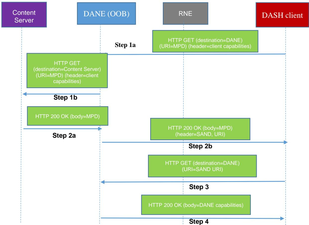
**Figure 4 - Workflow for client-triggered SAND capability exchange / negotiation with OOB DANE.**
