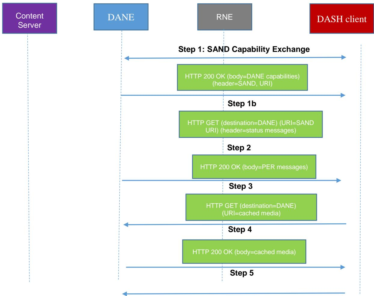
**Figure 8 – Another workflow for Proxy Caching for the case of advanced caching.**
