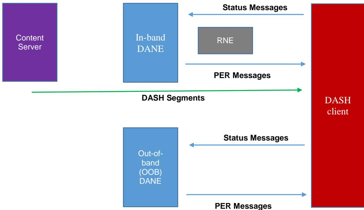
**Figure 2 – Assumed system architecture for SAND workflows**
