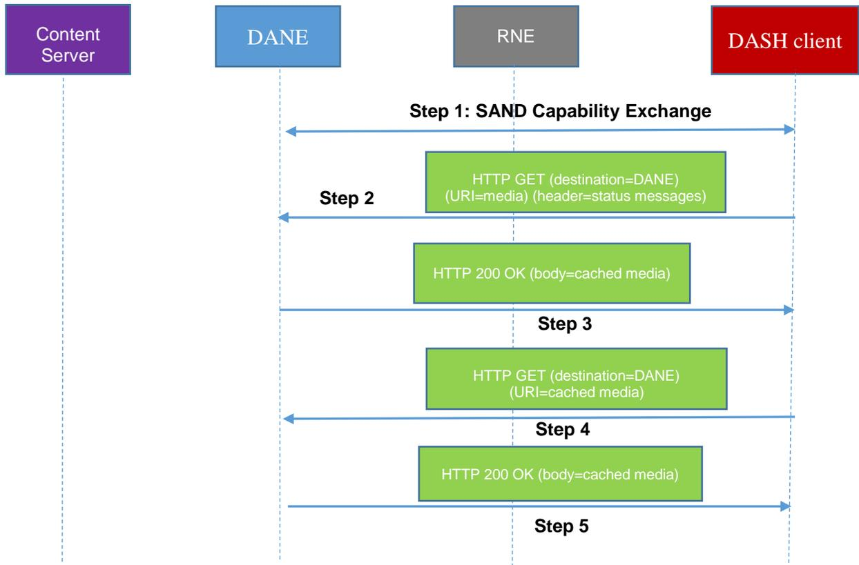
Figure 7 - Workflow for Proxy Caching for the case of advanced caching.
