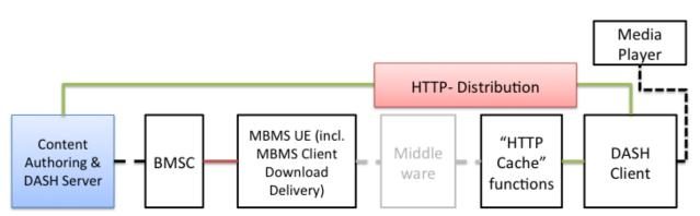
Figure 28 Typical Deployment Scenario for DASH-based live services partially offered through MBMS (unidirectional FLUTE distribution)
