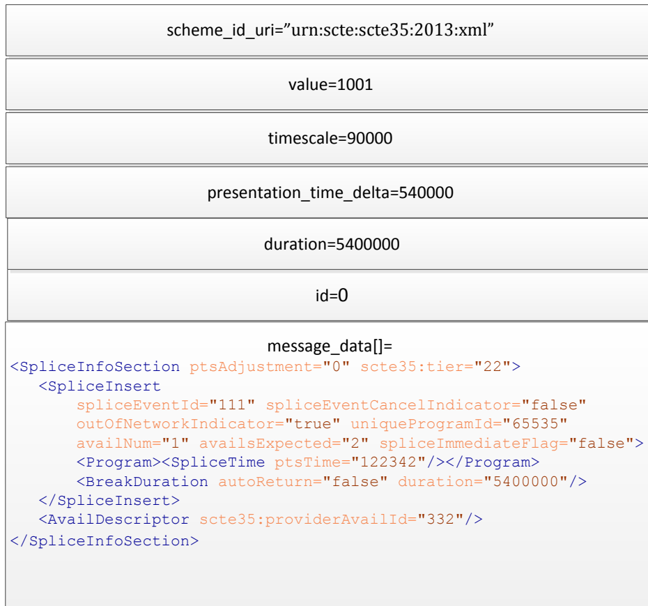
Figure 14 Inband carriage of SCTE 35 cue message
