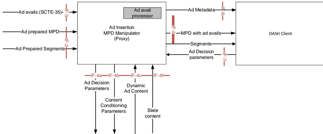
**Figure 6 MPD Manipulator Operation: Conforming IF-5 output**
